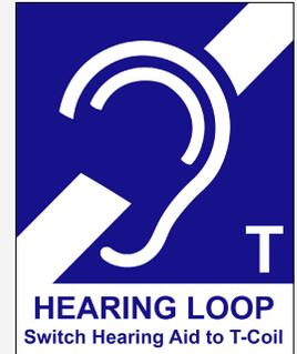
The Wisconsin Lutheran Synod has a useful bulletin on [Assistive Listening Devices](#). It also discusses "Hearing Loop" technology. They note, "A hearing loop provides a magnetic, wireless signal that is picked up by hearing aids/ cochlear implants set to the 'T' (Telecoil) setting. If hearing aids don't have a T-switch, a special receiver and headset are needed."
